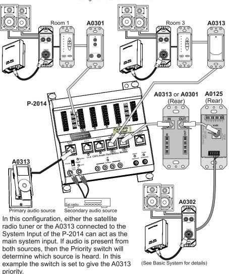
A0301 and A0313 can be used as primary system inputs feeding the main hub or as local input modules in each room to override the primary audio source. The A0301 is a generic input module which provides a standard L/R RCA input and the A0313 is an iPod® docking station.
