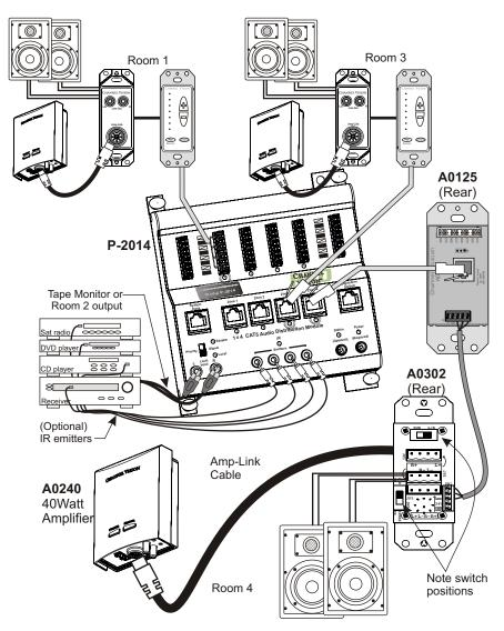
Most A/V receivers have a 'Tape Monitor' or 'Room 2' output that can be used to feed directly into the local input on the P-2014.
