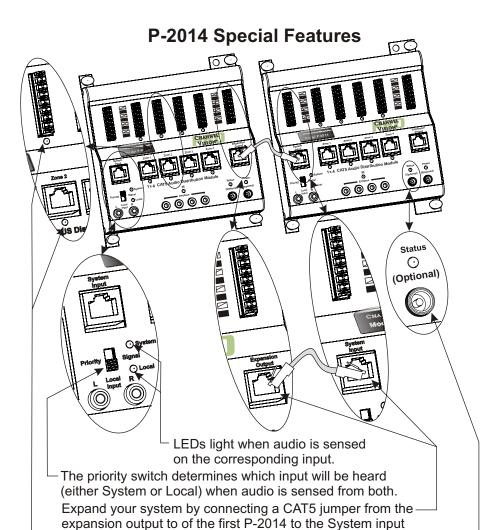
**Optional** Status power input senses when a connector is plug into it.— This connection has the potential to disrupt some of the automatic switching features built into the A0125 keypad. It exists for future uses only and potential applications will be described in future manuals.
