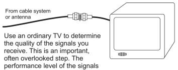
sets the standard of what you can achieve. If your signals are poor, try to correct them before you continue! This may mean complaining to your cable company, changing antennas, adding an antenna preamp or just aiming your antenna better. An RF distribution system will not improve the performance of the signals you start with!
