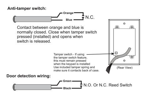
Alarm relay is activated upon Green - Black (ground) contact.
