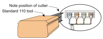
Caution: Be sure to use a standard 110 punch tool when connecting CAT5 wire to the 110 connectors. Using make-shift tools such as screwdrivers will cause the connector to become damaged and make the connection unreliable. Punch down as many as 4 incoming telephone lines on the input 110 punchdown as shown. Use a 110 punch-down tool to seat and trim all wires.
