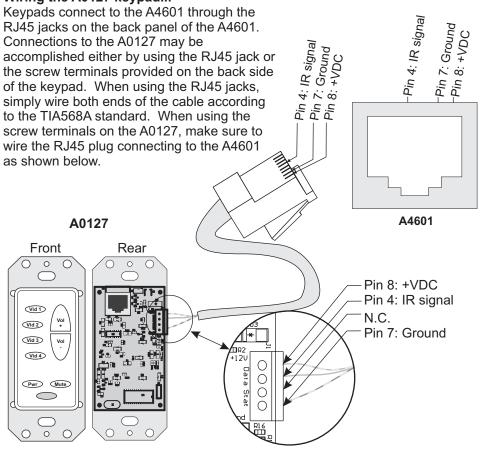
Connecting a standard IR repeater to the A4601... A standard IR repeating device may be connected directly to the A4601 allowing the unit to be controlled from a learning IR remote. The connection is similar to the wiring configuration shown above for the A0127, except there are only three wires as shown below.
