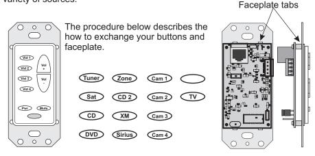
1 Detach the existing faceplate by pressing the plastic tabs with a flat blade screwdriver. (Press inward and upward ① at a 30 degree angle)
